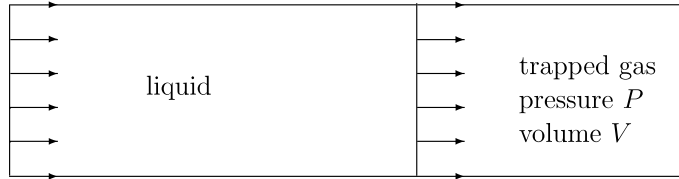
Fig. 18. Linear filling of a three-dimensional channel: two-dimensional cut. The interface moves with constant velocity v m/s.
